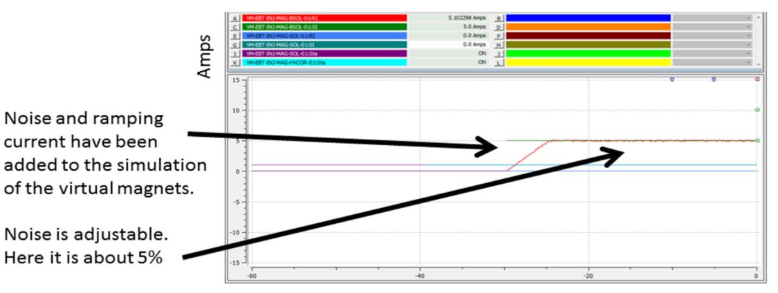
This is an example of a virtual magnet used to test a new Qt GUI striptool running under EPICSQt. The full online model is not needed here and just a basic set of magnet parameters are being simulated. Here the magnet current ramping, interlocks and noise are being generated in the virtual IOC. This tests was useful for rapid application development for CLARA GUIs
