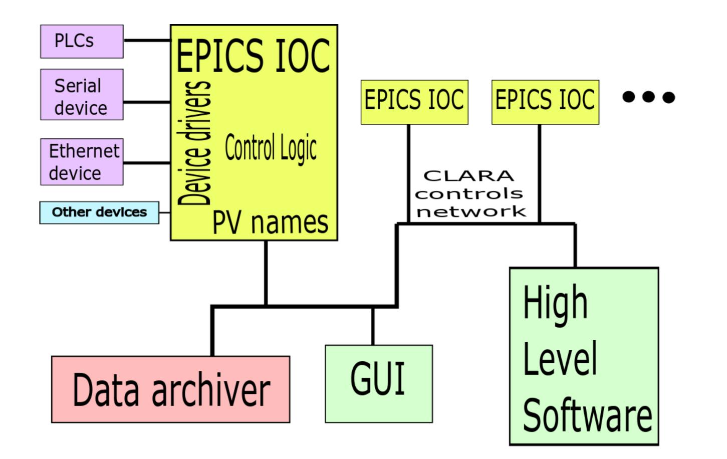
The CLARA technical sub-systems are managed within a distributed control system implemented with the EPICS software toolkit. The core of EPICS are IOCs that provide common controls over a network via Process Variables. A virtual accelerator has been made that simulates CLARA subsystems. The virtual PVs can be used without any particle tracking, providing simple functionality. In the case of magnets; current and interlocks. This mode has been used in the development of GUIs and State Machines.
