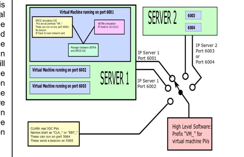
A virtual accelerator allows offline development of high level applications needed for the CLARA FEL to operate, these applications can be developed in parallel while CLARA is under construction and commissioning.
