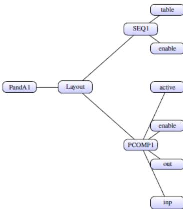
MalcolmJS must, therefore interrogate the attached device(s) for information on all the available function blocks, attributes and associated meta-data. The collection of internal resources then being listed in a "palette" in the right hand side-pane.
