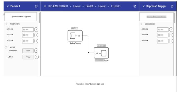
After checks for port type compatibility, the new association will be sent to the instrument, where the connection is made in internal logic. With the demand of high levels of user interactivity, it quickly became apparent that the user interface reactive, slick and intuitive.
