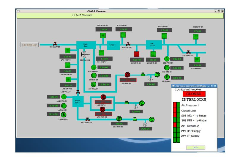
The status & interlocking system is responsible for on/off control and interlocking of hardware on the facility. It provides slow (>10ms) machine protection for technical sub-systems by only allowing operation of devices when predetermined conditions are met. It comprises of Omron CJ2M PLCs with digital I/O modules to marshal signals to and from hardware. ADC modules are also used to allow analog levels to produce interlocks directly within the PLC.
