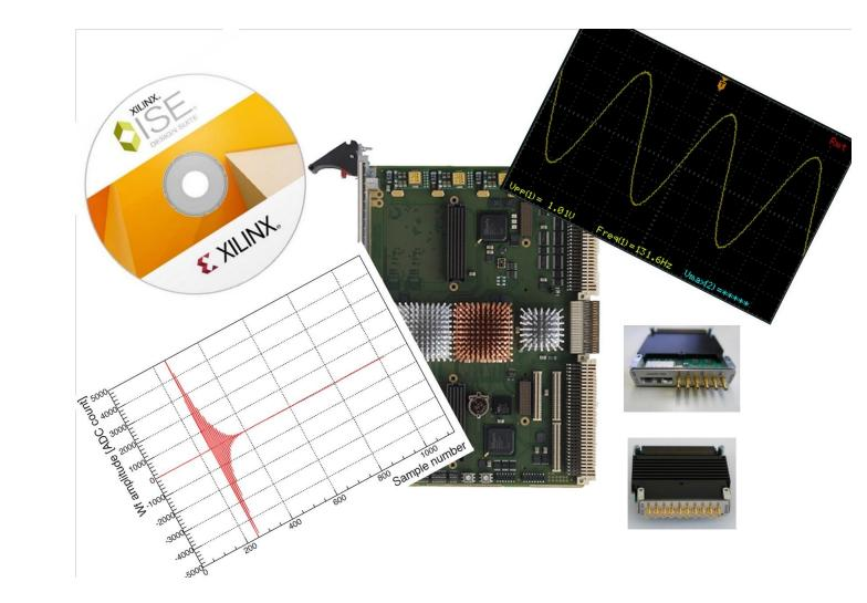
Stripline BPMs are digitised by a VME based system originally developed for EMMA. The system has been migrated the MVME5500/vxWorks from architecture of EMMA to the IOxOS IFC1210/Linux architecture for compatibility with the timing system. Diagnostic signals from cavity BPMs, bunch charge monitors, laser power meters and beam loss detectors will be sampled via systems using FMC data acquisition cards mounted on VME IFC1210 boards running EPICS.
