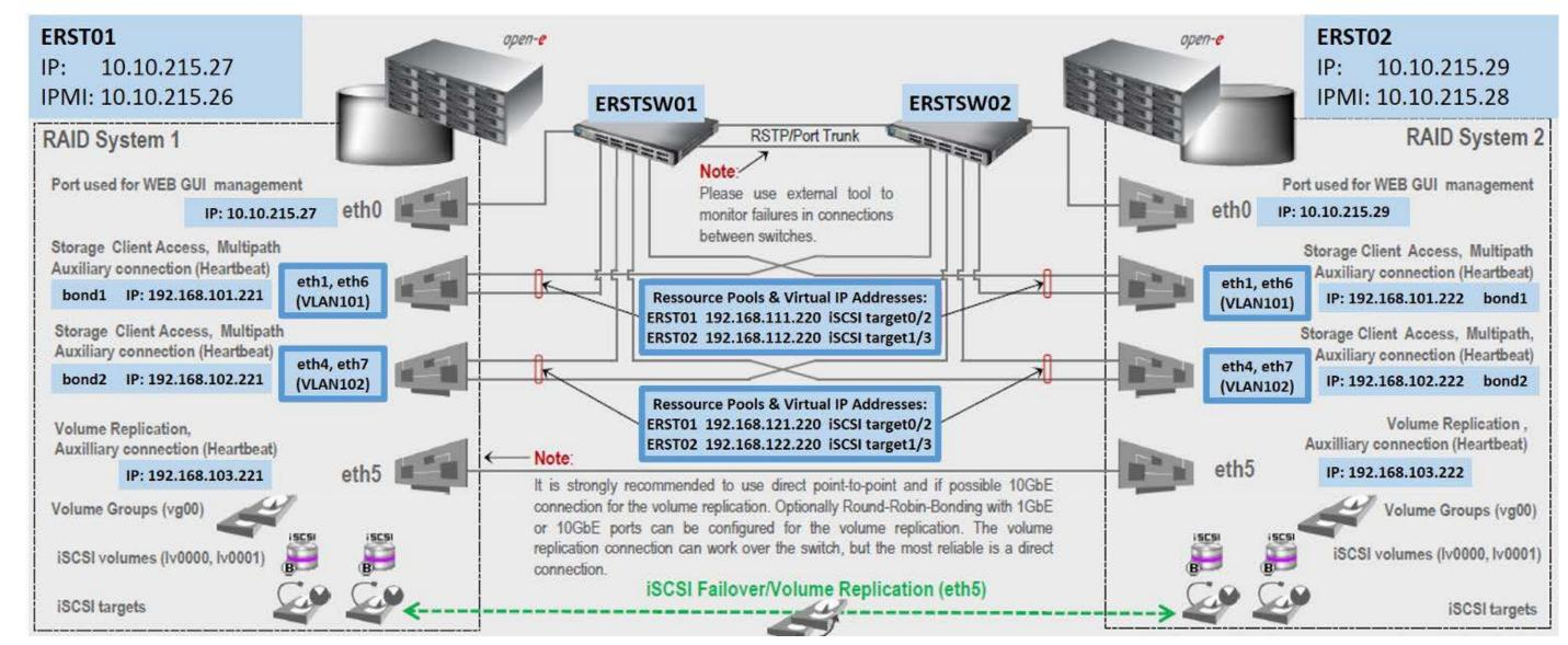
Fig. 4: Concept for the ACS Server Storage with 10GbE network iSCSI.
