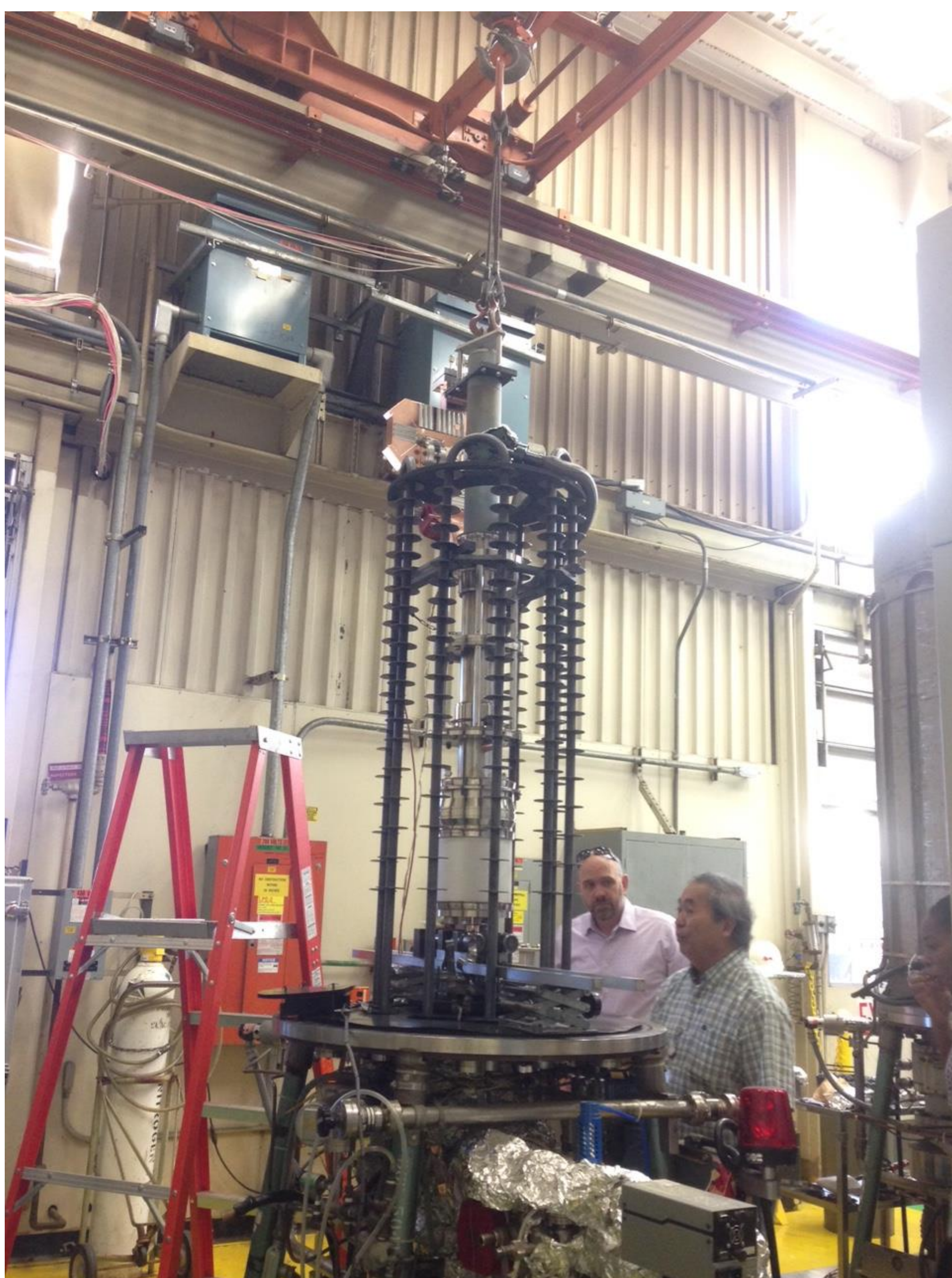
Bake Station 5 Oven with lid removed. Object mounted in center is a klystron preparing to be baked out.
