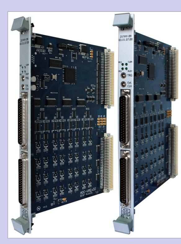
ADCx32 is the digitizer module that uses four 8 channel multiplexed 1 MSPS SAR ADCs with programmable channel sequencing. The sequence configuration determines sampling rate for each ADC channel individually.
