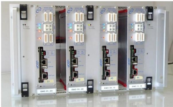
Figure 2: uSOP crate for BelleII monitoring system.
