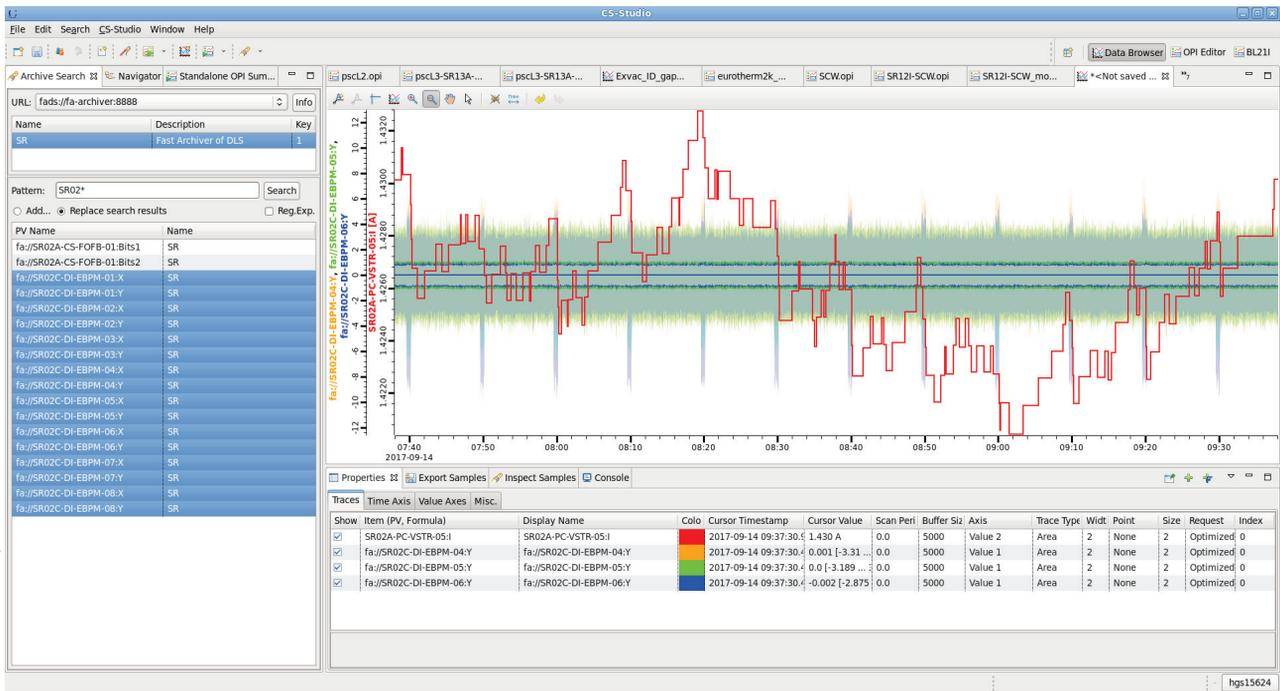
Figure 5: Databrowser plot showing EPICS archive data for a corrector magnet and fast archive data for nearby BPMs. The effect of the top-up process can be seen at ten-minute intervals.
