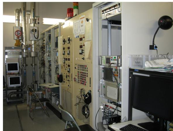
Figure 2: Photograph of the prototype LLRF system at the test stand.
