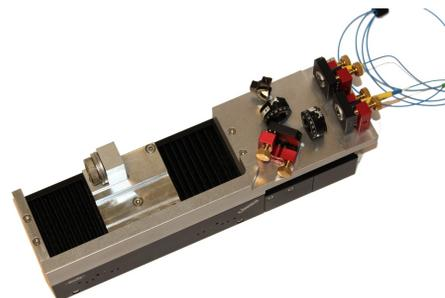
Figure 6: The delay stage is mounted on the linear stepper motor. For calibration purpose an encoder can be attached to the stepper motor as well (not shown in the photo).
