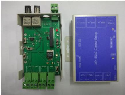
Figure 3: Photoelectric conversion module.
