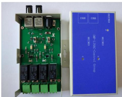
Figure 4: Relay module.
