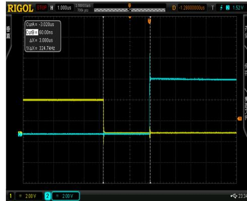
Figure 8: Fast chain protection system response time.
