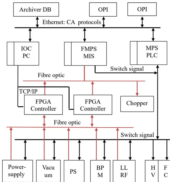
Figure 1: Injector II MPS system structure diagram.
