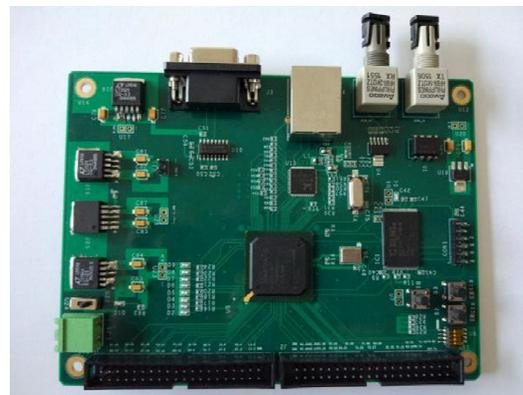
Figure 2: Front-end FPGA control board.
