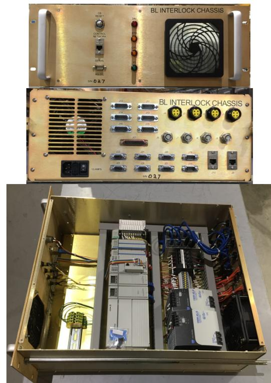
Figure 1: Intelligent Chassis Front/Rear Panel and Module Layout.
