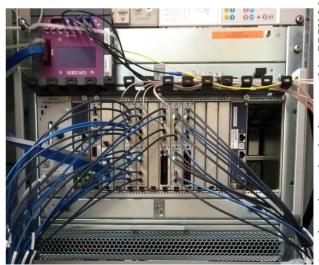
Figure 2: BPM DAQ system in μTCA form factor.
