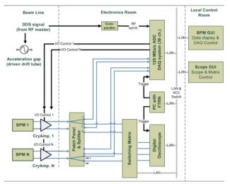
Figure 4: Schematic of the BPM signal chain and acquisition system.
