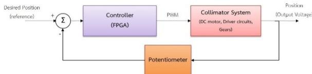
Figure 6: Feedback control loop of each collimator jaw.
