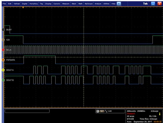
Figure 9: Interface signals between FPGA and ADC.
