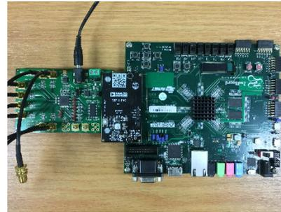
Figure 3: Zedboard and 8-channel ADC.
