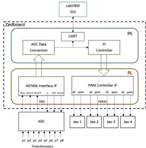
Figure 7: Block diagram of the control system and interface between hardware.
