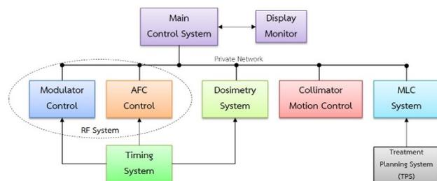
Figure 1: Network diagram of the machine prototype.
