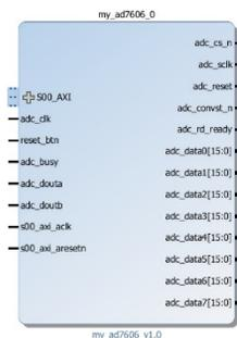
Figure 4: AD7606 Interface IP.
