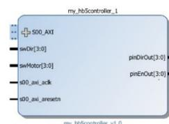
Figure 5: PWM Controller IP.
