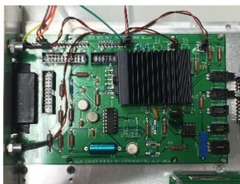
Figure 2: In-house PWM drive PCB.
