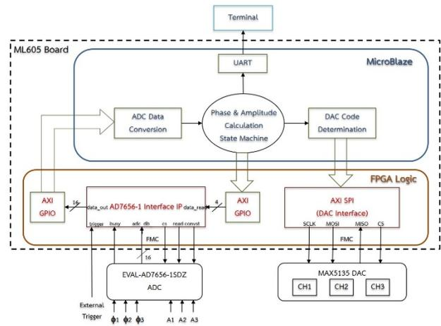
Figure 9: System block diagram for one ML605 board.
