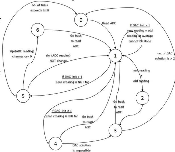
Figure 11: State machine diagram for phase calculation.
