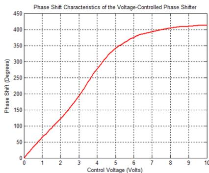
Figure 2: Typical phase shift characteristics of voltage-controlled phase shifter.
