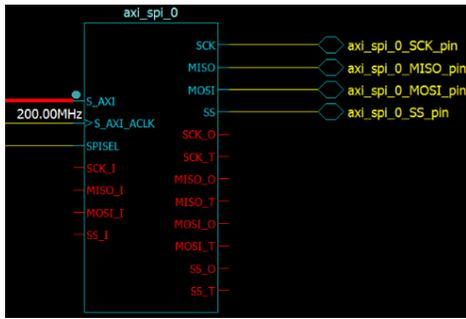
Figure 8: AXI SPI interface to MAX5135 DAC in EDK.
