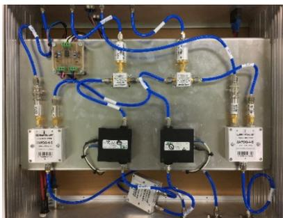
Figure 3: RF chassis of the phase and amplitude detector.
