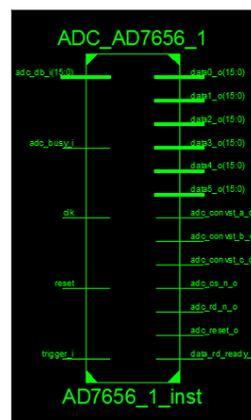
Figure 5: AD7656-1 driver IP with trigger input.
