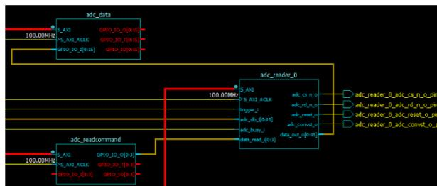
Figure 6: AD7656-1 Interface IP in EDK.
