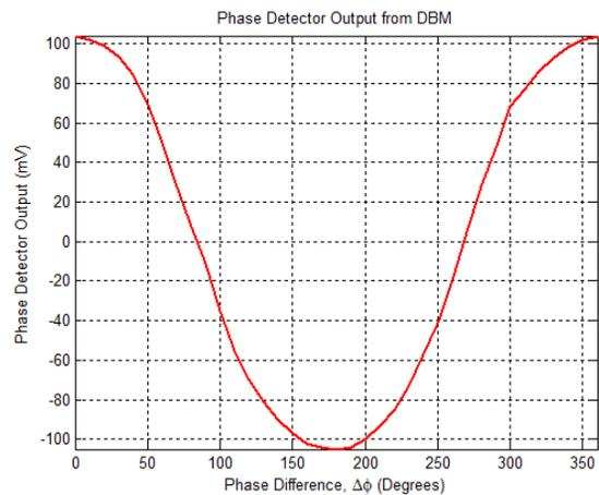
Figure 10: Phase detector output of the DBM.
