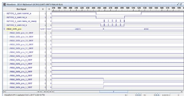
Figure 12: Interface signals and data bus between FPGA and ADC.
