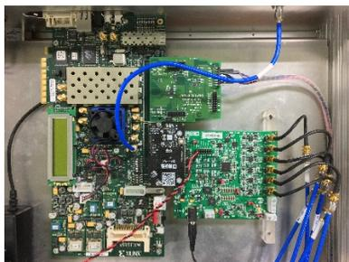
Figure 4: Virtex-6 ML605 FPGA board with AD7656-1 and MAXSPCSPARTAN6+ daughter boards.
