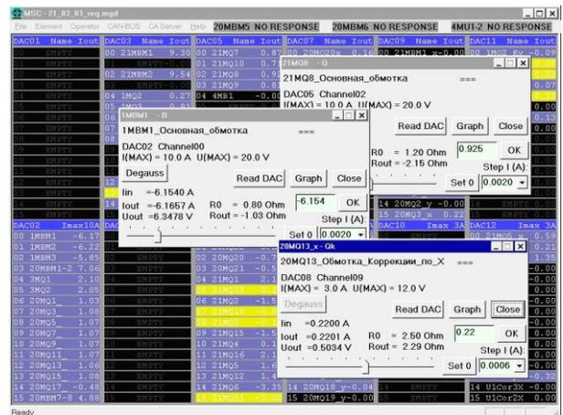
Figure 5: FEL magnetic system control application.
