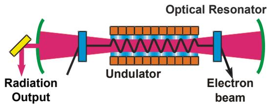
Figure 2: FEL operation principle.
