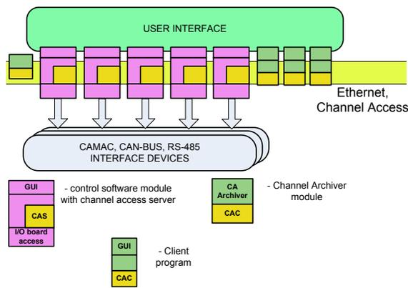
Figure 4: Architecture of FEL control software.
