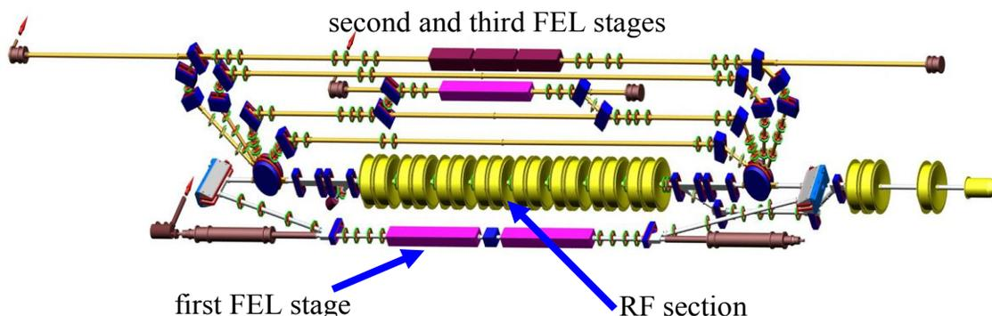
Figure 1: Multi-turn accelerator-recuperator of Novosibirsk FEL scheme.
