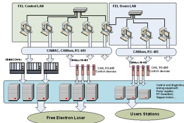
Figure 3: FEL control system hardware.
