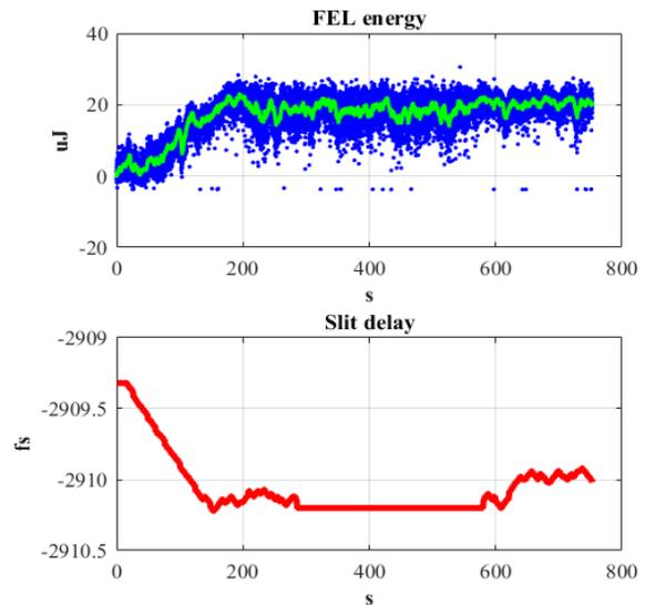
Figure 3: Example of automatic optimization of the delay between the seed laser pulse and the electron bunch using the correlation minimizer acting on the delay line. After reaching the maximum the minimizer is turned off. At 580 s the minimizer is switched on again in “balanced search” mode which decreased the FEL energy *rms* from 16% to 10%.
