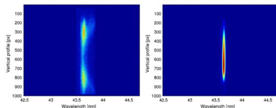
Figure 6: FEL spectrum before (left) and after (right) optimization based on the *FELQFactor* index. The horizontal axis in the images is the photon energy, while the vertical axis represents the vertical photon beam distribution.
