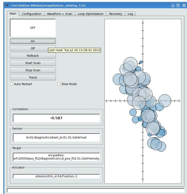
Figure 2: Graphical interface of the correlation minimizer. The spots on the right represent the relationship between the target (vertical axis) and the sensor (horizontal axis). The spots are big for the most recent samples and get smaller as the samples become older. In the example of the figure the correlation is almost linear and the correlation index is -0.587.
