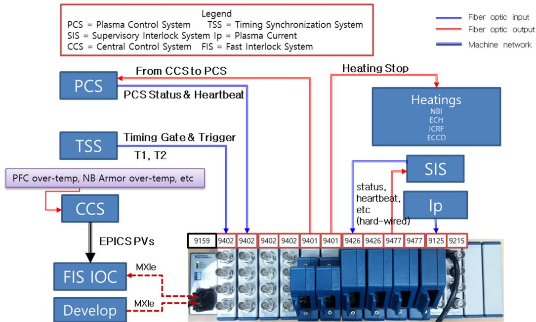
Figure 1: Configuration of KSTAR fast interlock system.
