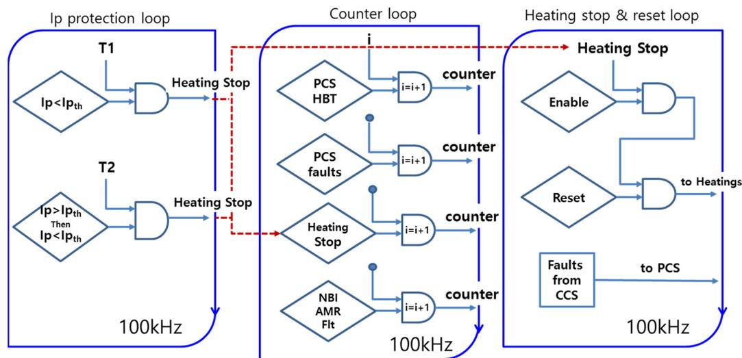
Figure 3: FPGA logs for three independent loops.
