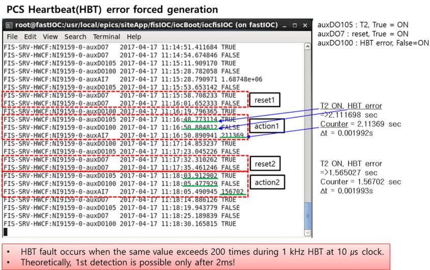
Figure 2: Functional operation test result for the PCS heartbeat error counter.
