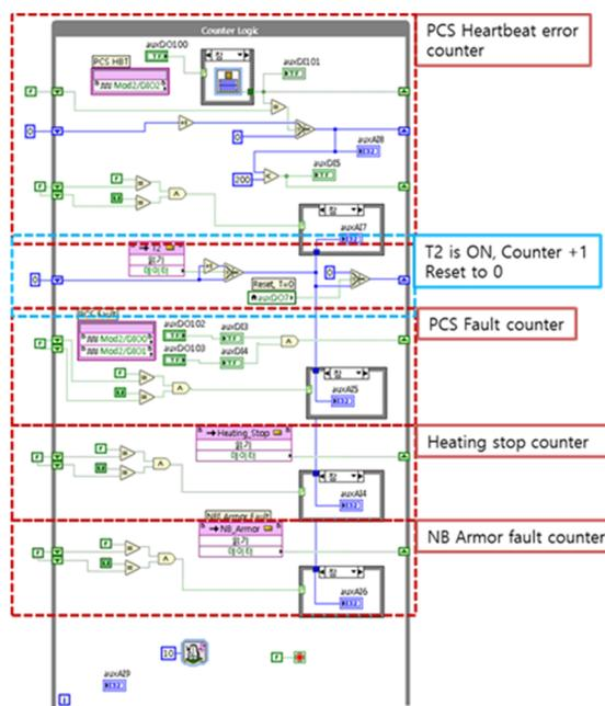
Figure 2: LabVIEW FPGA code for the counter logic.
