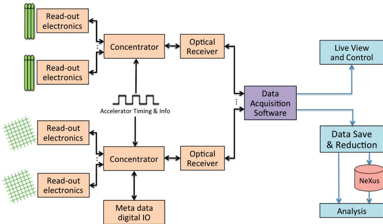
Figure 1: Data Acquisition System components at SNS
