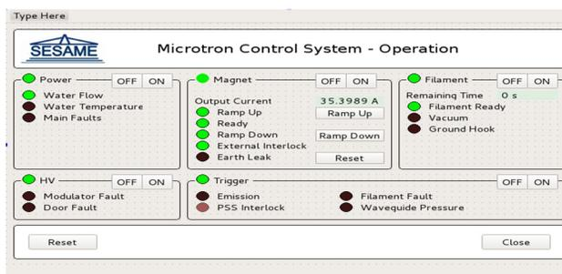
Figure 5: Microtron control system in Qt framework.
