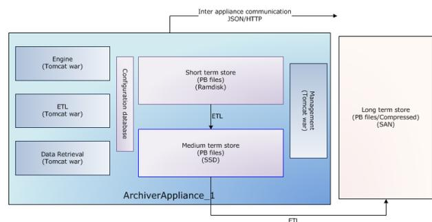
Figure 7: Architecture of a single appliance.
