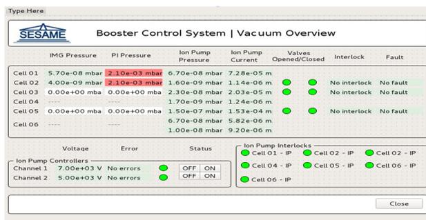
Figure 6: Booster vacuum control in Qt framework.
