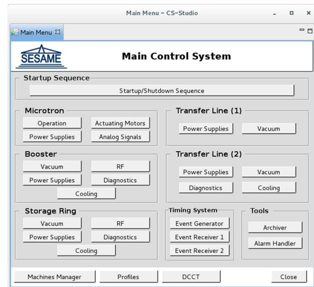
Figure 1: Main interface for the control system client.
