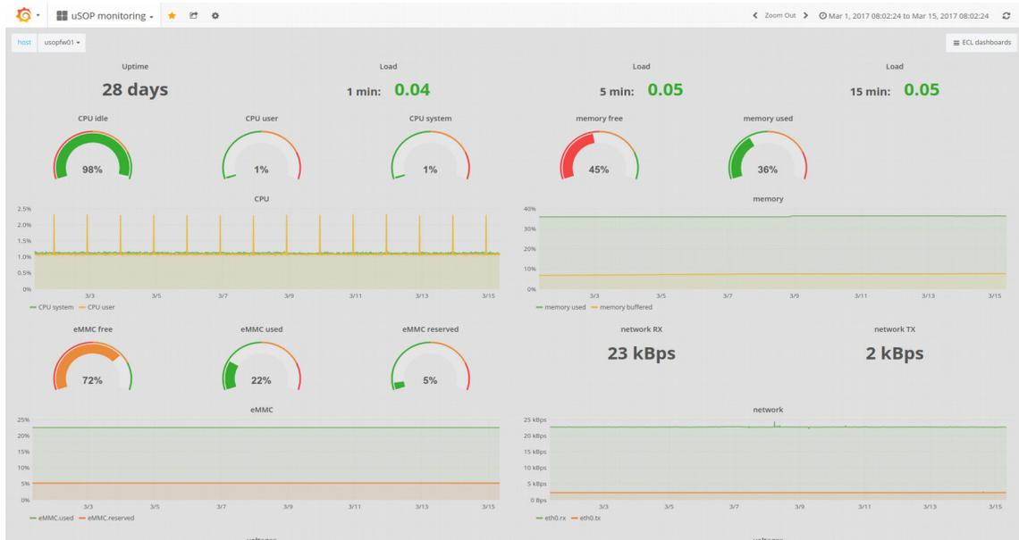
Figure 3: uSOP dashboard for system metrics monitoring.
