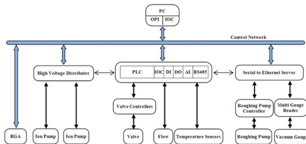
Figure 1: Block diagram of vacuum component and related controller.
