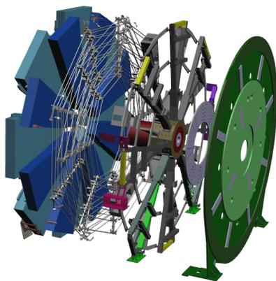
Figure 1: An exploded view of the NSW. From left to right: The detector sector envelopes, the alignment system, the structure and the New JD (shielding and support).
