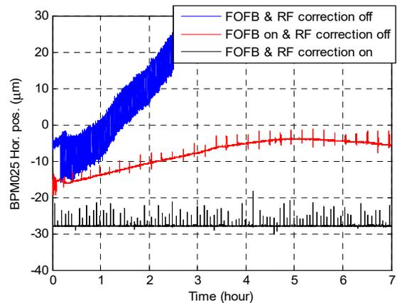
Figure 8: Orbit stability comparison with/without FOFB and RF path length compensation. The spikes are due to regular injection when FOFB and RF frequency correction is temporarily inactive.
