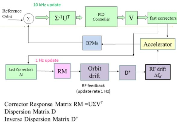
Figure 7: FOFB with RF correction (schematic).
