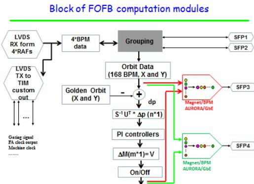
Figure 3: Functional block of FOFB computation module.
