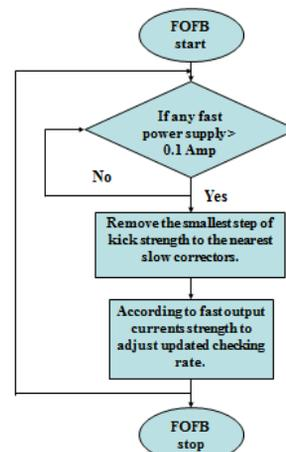
Figure 6: FOFB with slow corrector compensation to avoid fast corrector saturation.
