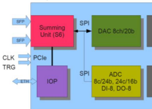
Figure 4: There are four major modules inside Corrector Power Supply Controller (CPSC): IOP, ADC unit, DAC unit and FPGA for FOFB fast setting.
