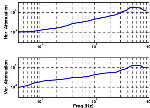
Figure 5: The measured bandwidth of FOFB. Horizontal is around 250Hz and vertical around 300 Hz.
