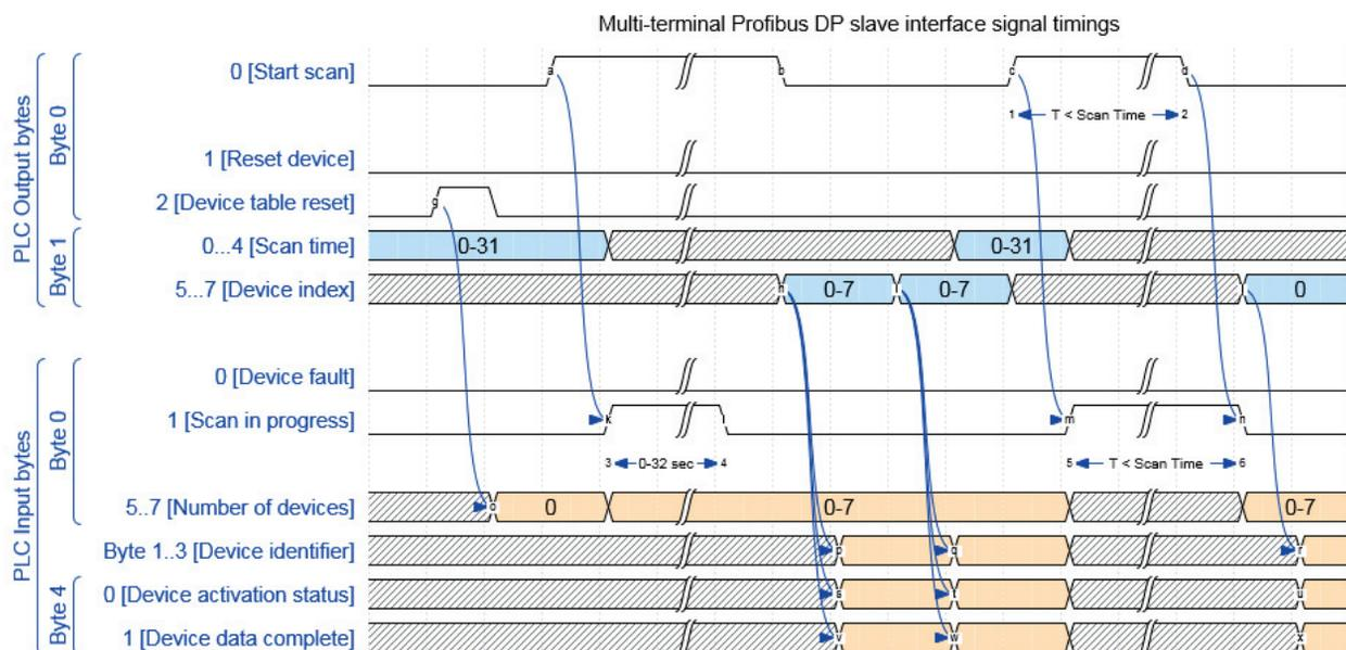
Figure 3: PLC output and input signal timing diagram.
