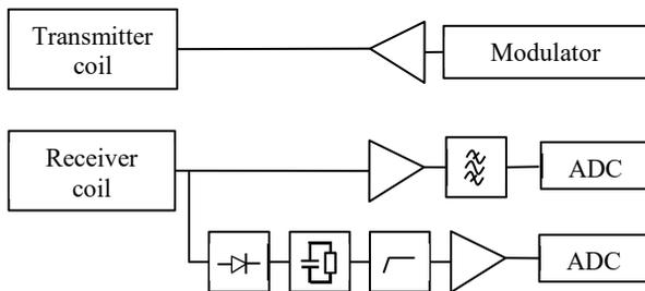
Figure 2: Block diagram of the antenna and the frontend.
