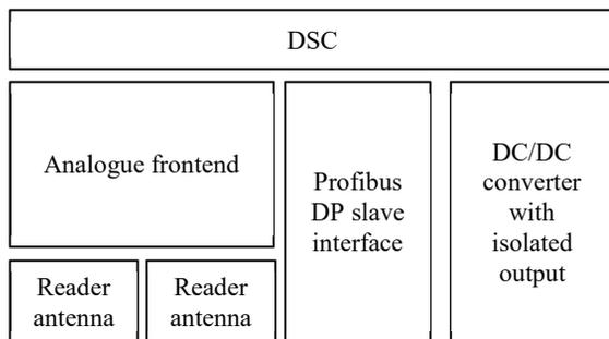
Figure 1: Architecture of the terminal device.
