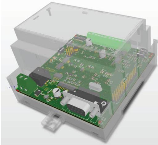
Figure 4: The multi-protocol terminal in a DIN-rail compatible enclosure.
