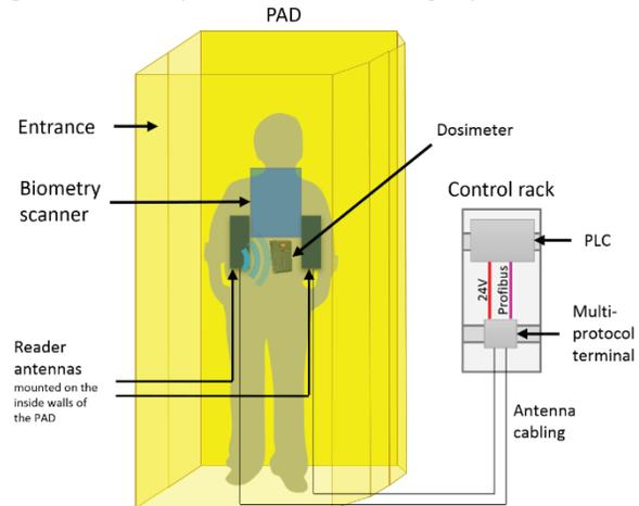
Figure 5: Integration of the terminal unit inside a PAD.
