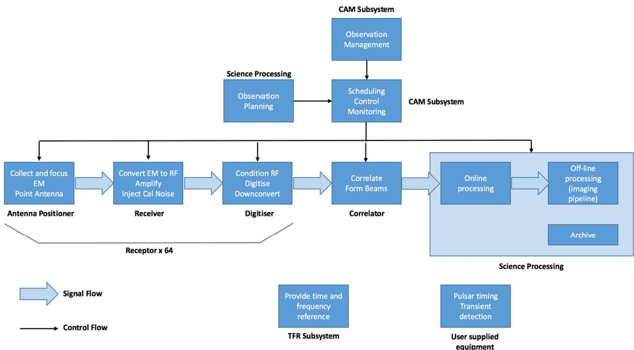
Figure 1: Functional view of the MeerKAT Telescope system [4].
