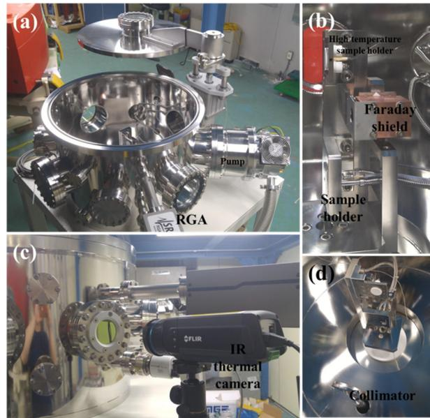
Figure 8: Pictures of (a) the beam target chamber, (b) the sample holders, (c) the IR thermal camera, and (d) the collimator.
