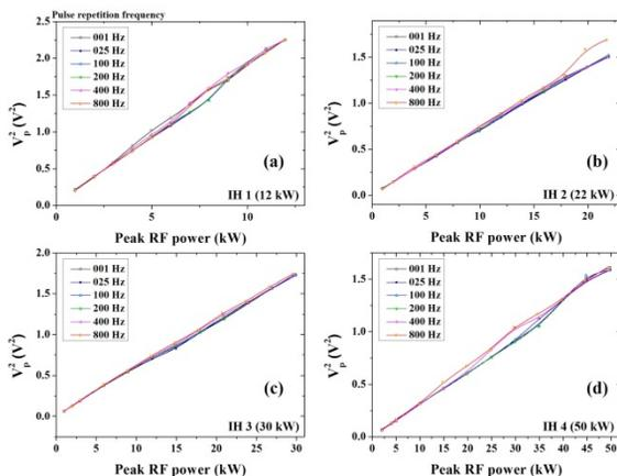
Figure 2: The values of squares of RF pickup loop voltages in the (a) IH1, (b) IH2, (c) IH3, and (d) IH4 tanks as a function of peak RF power.
