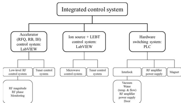
Figure 4: Schematic diagram of DIAC integrated control system.
