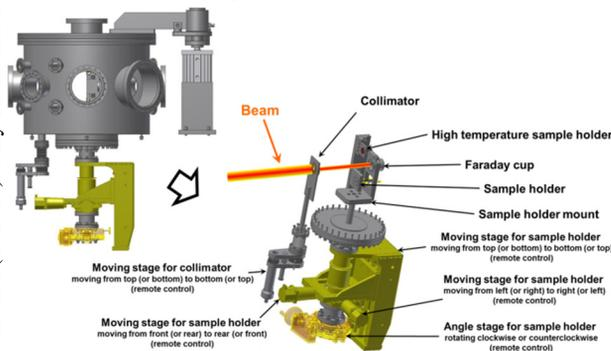
Figure 7: A 3D sketch of the beam target chamber and various diagnostic systems.
