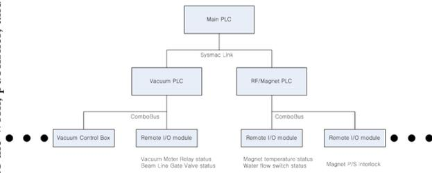
Figure 6: Schematic diagram of the DIAC interlock system.
