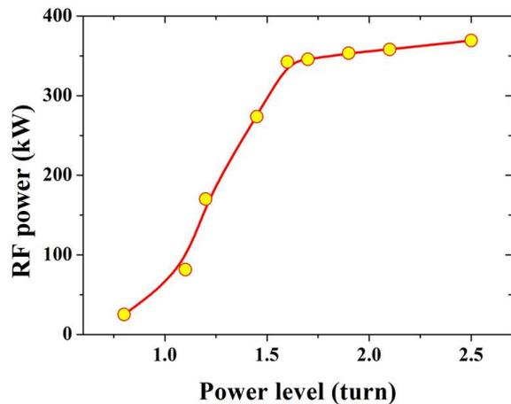
Figure 3: The applied RF power as a function of power level in the RFQ RF amplifier.
