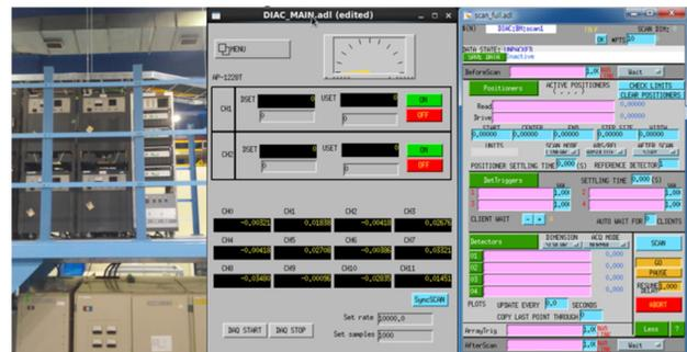
Figure 5: Power supplies and EPICS based control system for electromagnets.
