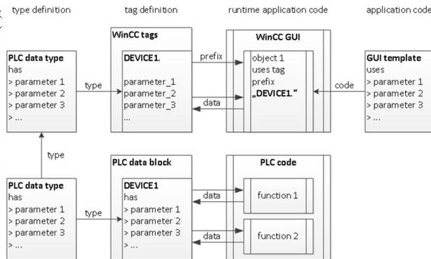
Figure 2: PLC and WinCC object oriented data handling.
