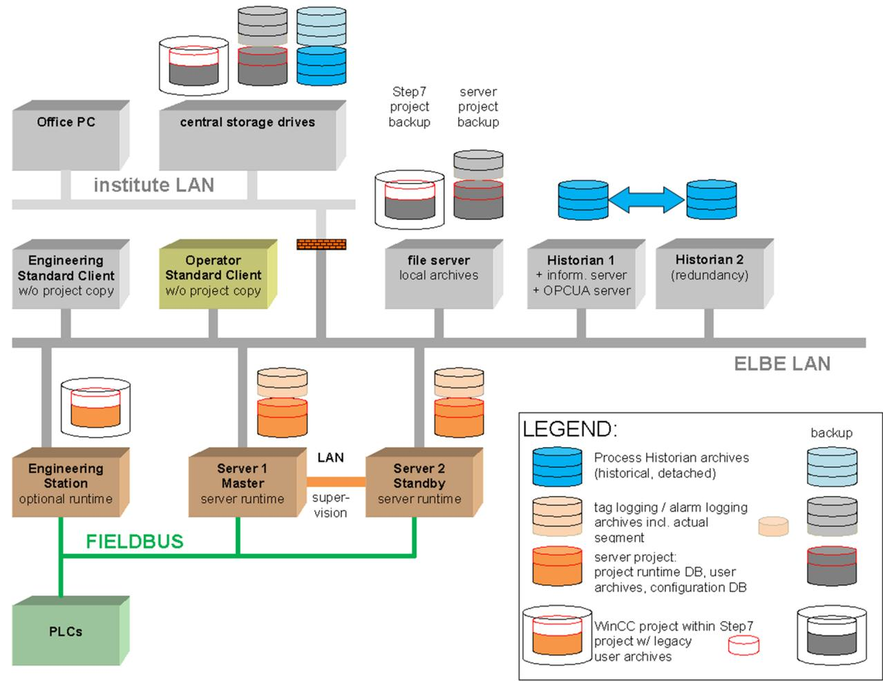
Figure 3: The new WinCC system architecture.
