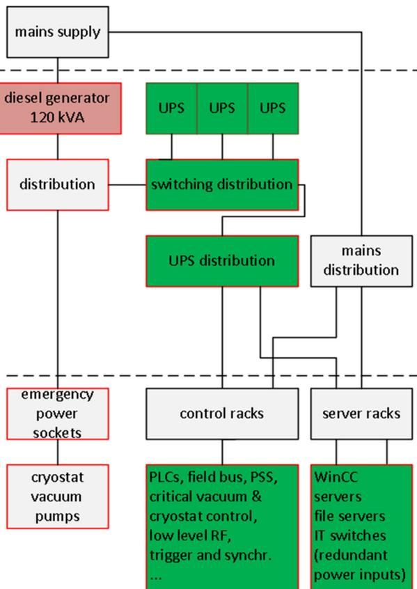
Figure 4: Electrical infrastructure for control system related components.
