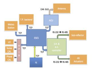
Figure 2 Block diagram describing DISCOS installation (ESCS) and customization for Noto radio telescope
