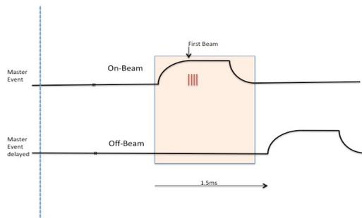
Figure 1: Timing shift of the RF pulse.
