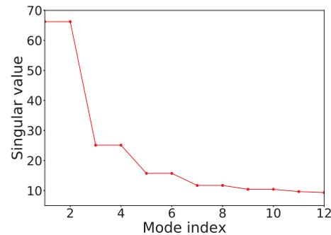
Figure 3: Singular values of simulated SIS18-ORM in y-plane.
