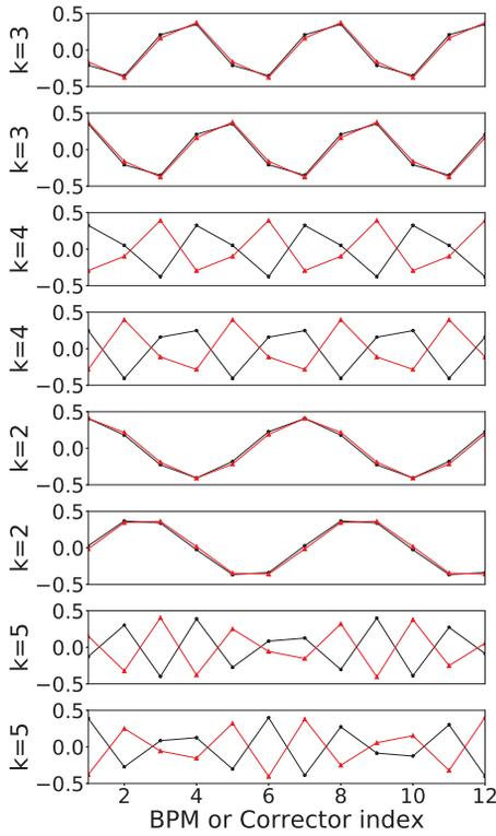
Figure 4: Columns of  $\mathbf{U}$  (black) and  $\mathbf{V}$  (red) matrices generated by SVD of simulated SIS18-ORM in y-plane.
