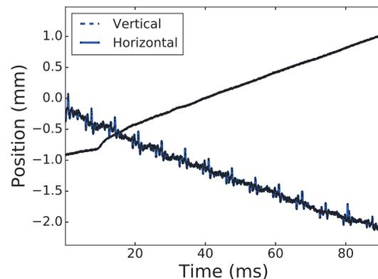
Figure 1: Position in both planes measured at BPM in section 8 during first 90 ms in the acceleration ramp.
