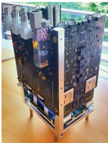
Figure 2: Stripped GigaFRoST camera. Visible are one readout board and the control board with BNC connectors and single Ethernet connection.
