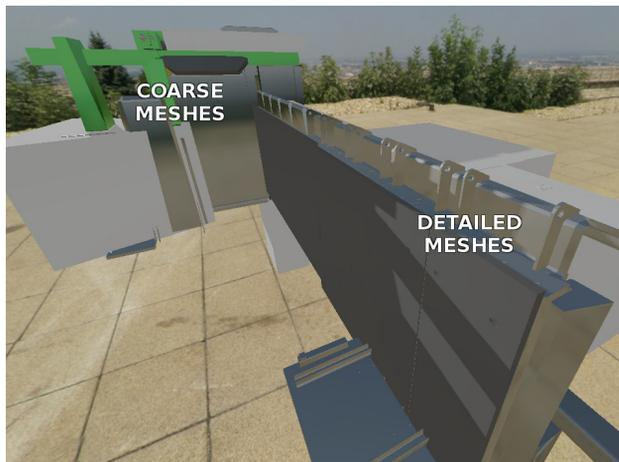
Figure 8: Screenshot of the Viewer showing the LODs depending on the distance from the point of view.
