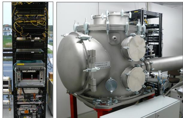
Figure 4: Test-bed Control/DAQ rack, vacuum test system.
