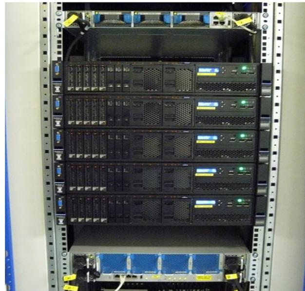
Figure 6: Control Servers, also visible: TOR- and BOR-Switches.
