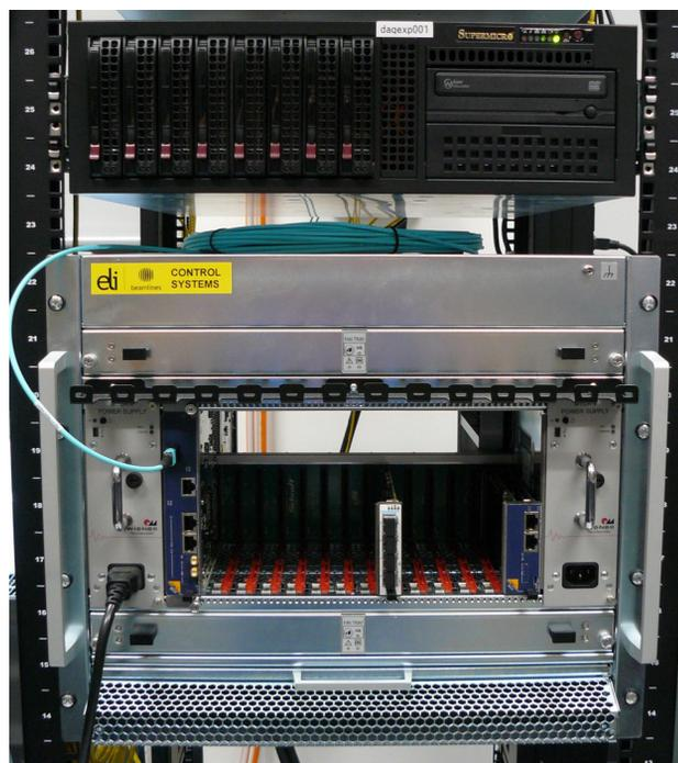
Figure 8: Standard PCIe DAQ system (top) connected with MTCA DAQ system (bottom) via optical fibre / PCIe bus
