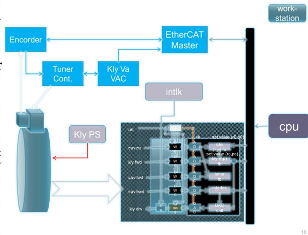
Figure 5: Schematic of RF test stand with MTCA.4 and EtherCAT.
