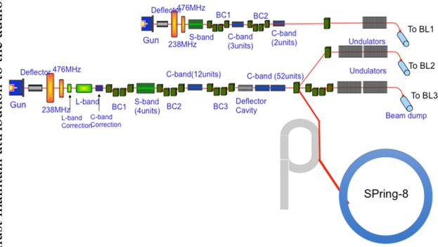
Figure 2: Schematic drawing of the SPring-8 accelerator complex.
