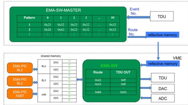
Figure 6: Schematic of bunch by bunch parameter control.
