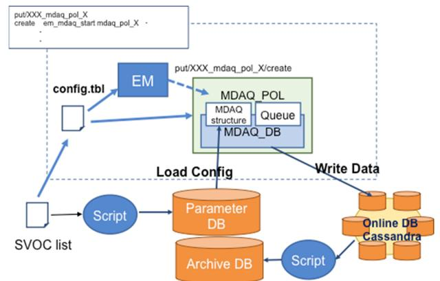
Figure 4: Schematic of the data acquisition framework. This shows a point data acquisition scheme to be polling.
