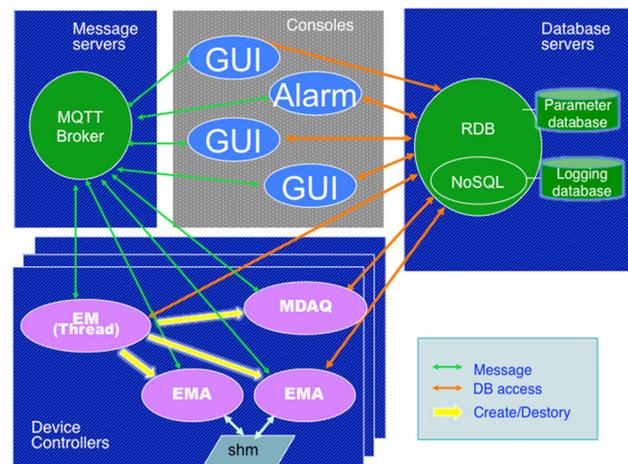
Figure 3: Schematic of the control framework for the SPring-8 accelerator complex.
