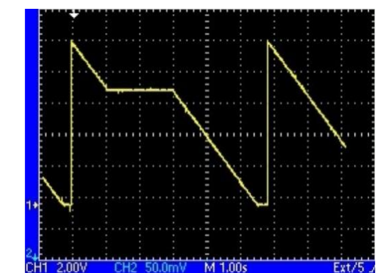
Fig. 2: Test of a redundant configuration based on "software backup". Master to Reserve switching takes 2 secs (Processors: Siemens S7-315DP)
