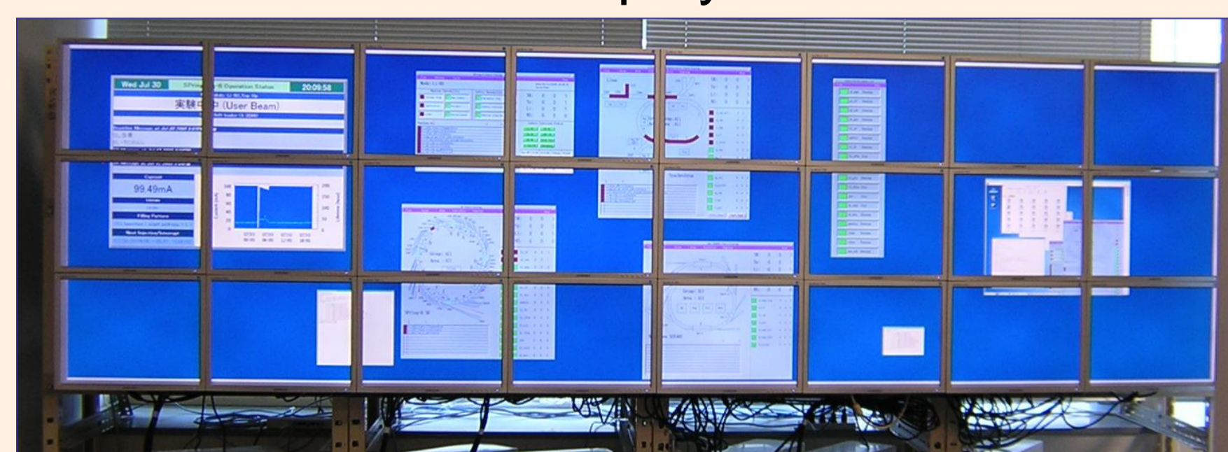
Twenty four LCD panels SAMSUNG SyncMaster 204B • 20.1 inch • 1600 × 1200 pixels
