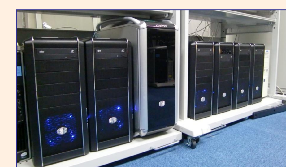
Display wall machines • CPU: Intel Core i7 2.93GHz • Memory: 8GByte
