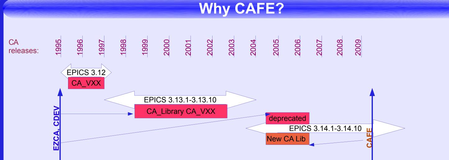
Modest changes to channel access (CA) over the past many years safeguard compatibility between old and new client/server connections. However, many C/C++ extensions (or wrappers) to CA are either frozen or not rigorously maintained and often do not reflect recent advances in channel access, such as multithreading and handling of lost connections.
