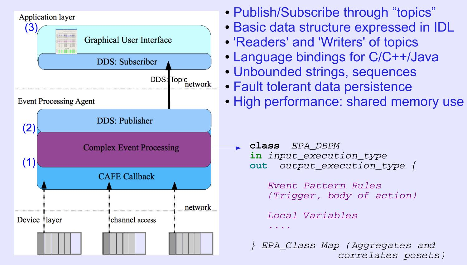
(1) The Event Processing Agent (EPA) is configured from XML and uses the CAFE API to establish a callback mechanism to EPICS
