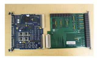
Figure 1: Control card and break out board.
