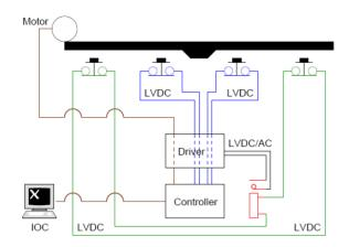
Figure 3: Independent limit switch scheme.
