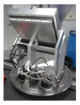
Figure 4: Far-IR mirror mount with motors.
