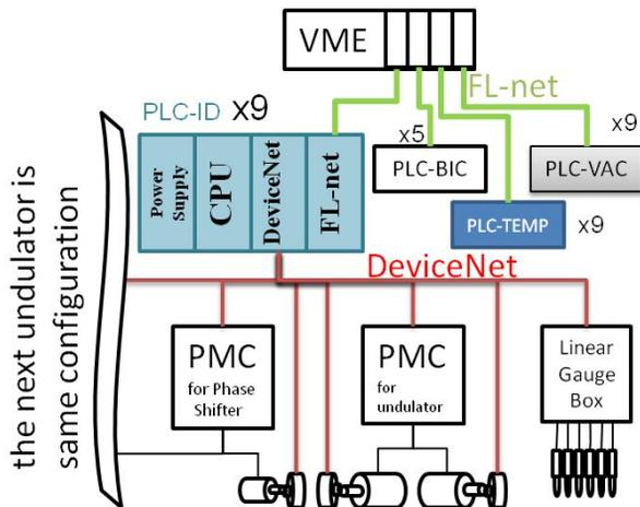
Figure 3: Schematic of PLC and control devices.
