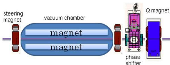
Figure 1: Configuration of undulator system.
