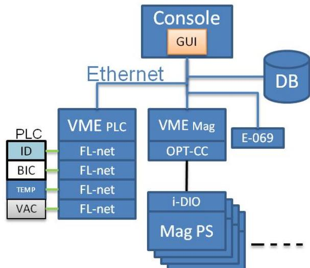
Figure 2: Schematic of ID system.
