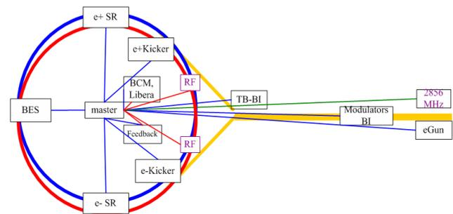
Figure 1: Layout of BEPC-II timing system stations.
