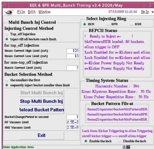
Figure 3: Top-off injection control OPI.
