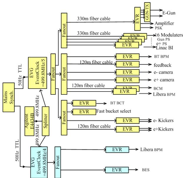
Figure 2: Logic connections of BEPC-II timing system.
