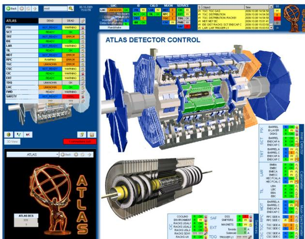
Figure 2: ATLAS FSM operator interface.
