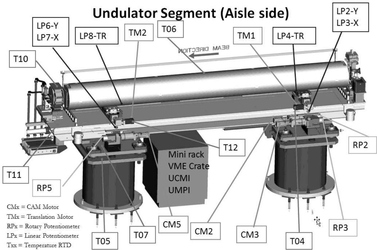
Figure 1: Undulator controls equipment, aisle side.
