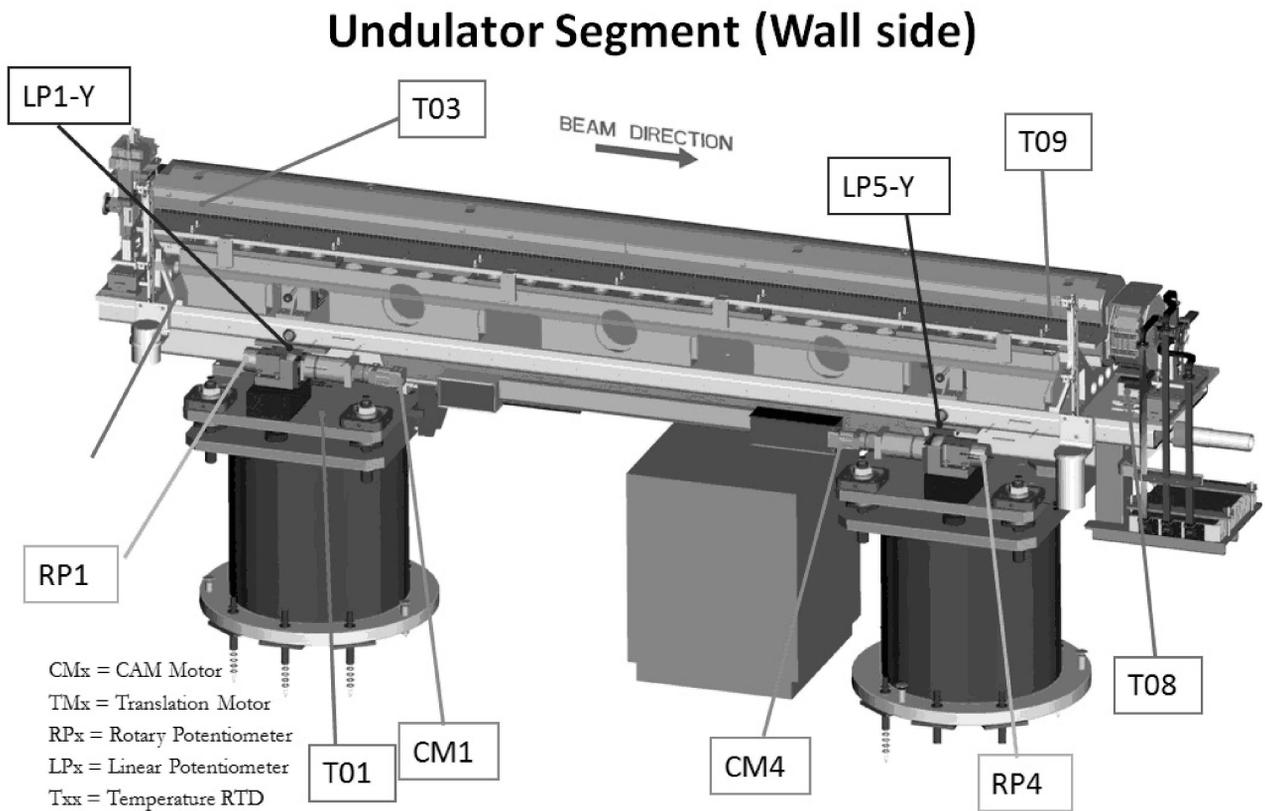
Figure 2: Undulator controls equipment, wall side.
