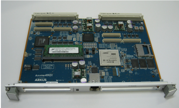
Figure 2: Photograph of upgraded base board of the flexible logic-reconfigurable VME board. PCI bus interface (upper left) and gigabit Ethernet port (bottom) facilitate fast data transfer.
