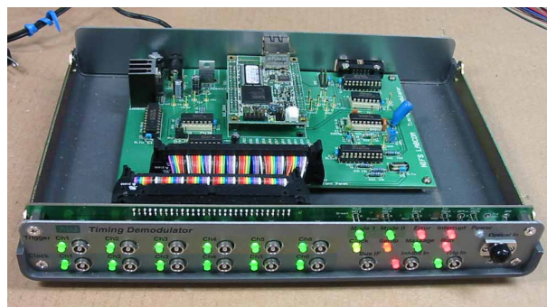
Figure 6: Front and inside view of newly developed FPGA demodulator box: The central small piggyback module is Atmark Techno's Suzaku-S (SZ130).
