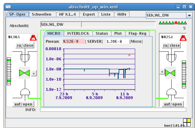
Figure 4: PETRA vacuum controls displaying DOOCS and TINE data.
