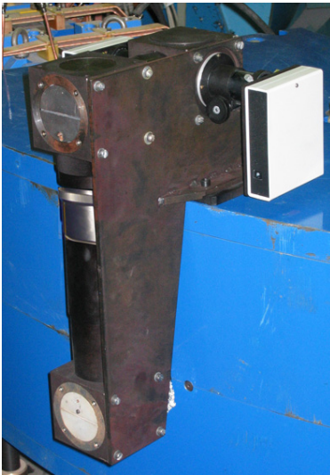
Figure 2: Optical bench with system of movable mirrors and SR diagnostic station with two CCD cameras.
