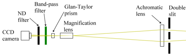
Figure 3: Schematic drawing of the SR interferometer.
