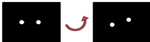
Figure 2: Determining changes in alignment from the position of the received flashes from two BCAM diodes.
