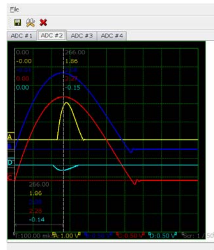
Figure 6: Digital oscilloscope application. There are four pulses of different elements of injection channels.
